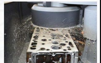
Wet surface grinding
