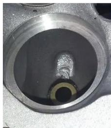
Cam bucket bore machining
