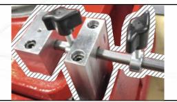
Adjustable travel stop system on the sliding plate to ensure the operator doesn't contact the valve stem with the wheel edge.
