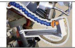
Integration of the flexible hose on the on the valve support unit, allowing to keep a consistent collant flow over the valve
