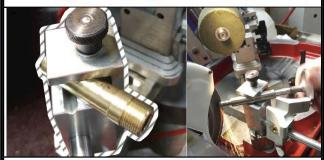
New universal support allows mounting of valve guides to regrind valve tips more accurately than before.
