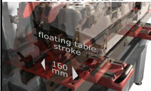
Cylinder heads up to 350 kgs can be moved back and forth without any effort and then locked by two powerful pneumatic jacks.
