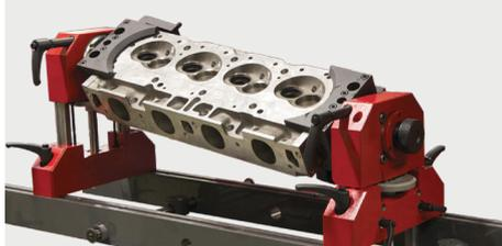
Heads with tilted or canted valve guides can be positioned quickly, even if sides are parallel or not. Set the cylinder head at the desired level and roll it over. Sturdy clamping thanks to two large jaws. Sphere centering handles to get a quick mount of the head. Firm locking of the jaw's shafts through two handles for a perfect clamping while machining.
