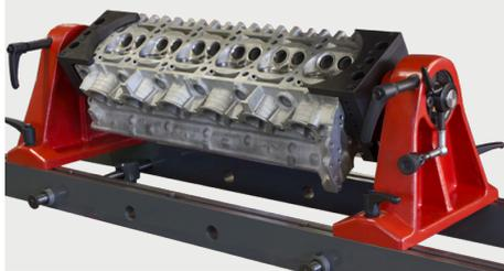
Allows quick positioning of parallel and non-parallel side heads with tilted valve guides. Sturdy clamping thanks to two large jaws. 360° rotation to get an easy access to all sides of the cylinder head for various jobs. Firm locking of the jaw's shafts through two handles for a perfect clamping while machining.
