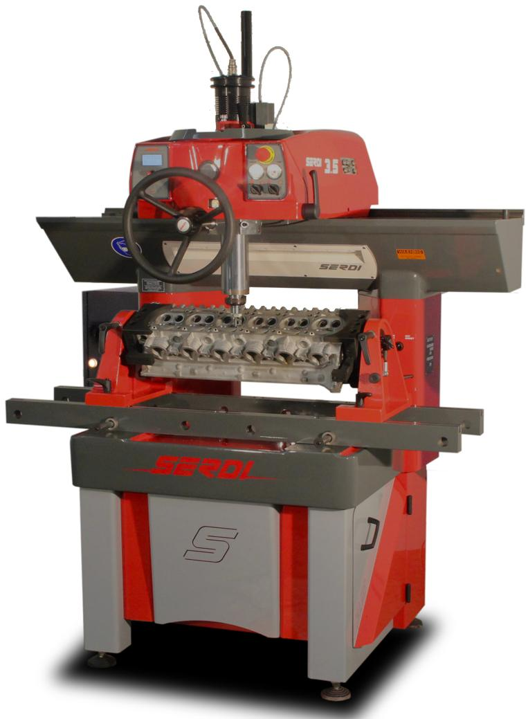
High precision valve seat and valve guide cutting machine especially designed for multi-valve cylinder heads.
