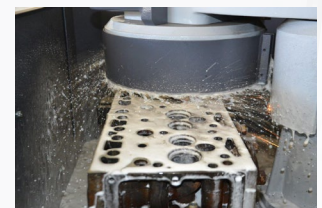
Wet surface grinding
